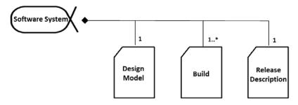
Figure 9.45 - Software System Alpha and three Work Products: Design Model, Build, and Release Description with visualized bounds
