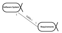
Figure 9.28 - Alpha Association between the Requirements Alpha and the Software System Alpha, read as: "The Software System fulfills the Requirements."
