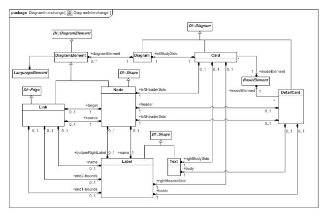
Figure 9.23 - Metamodel of the graphical syntax for diagram interchange
