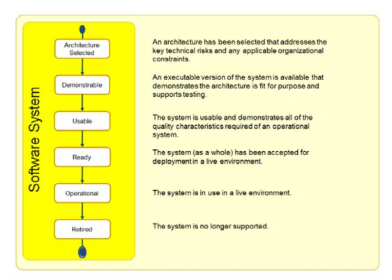
Figure 8.8 - The states of the Software System
